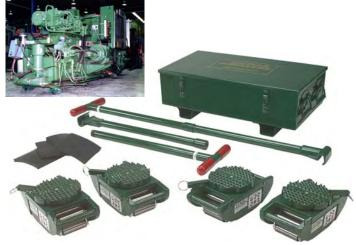
Easy and safe to use! Just lift the load, set the Rollers, and move. The recirculating chains on the Hilman Rollers provide controllable heavy moving right on ordinary flooring. Fully directional swivel tops allow equipment positioning in the tightest quarters. 3 and 8 ton Kits and Sets feature swivel padded rollers. 15 ton and higher Kits and Sets are available with your choice of swivel-locking padded rollers or rollers with swivel-locking diamond steel grid tops and loose Preload Pads.
